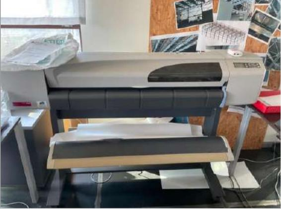
A large-format HP DesignJet 500 plotter is shown in an office setting. It is a wide, flatbed printer with a paper tray on the left and a collection tray on the right. The machine is primarily white with black accents.                                                        |
